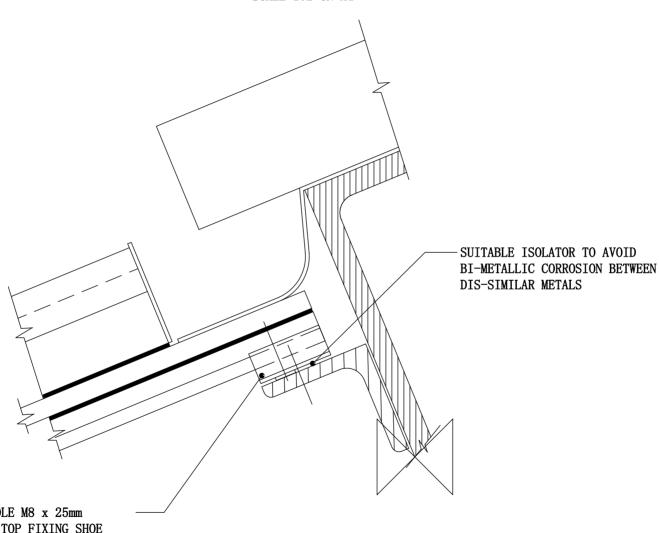
SINGLE HOLE M8 x 25mm POSITIVE TOP FIXING SHOE RIVETTED TO BAR
