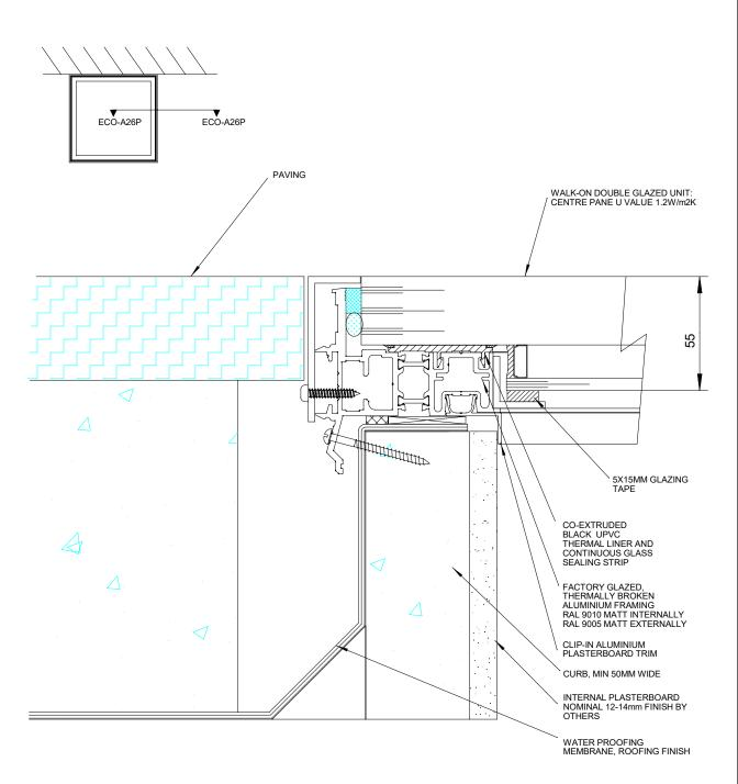
CONCENTRATED LOAD MUST NOT EXCEED 2000 N AND UNIFORM DISTRIBUTED LOAD MUST NOT EXCEED 2500  $\rm N/m^2$
